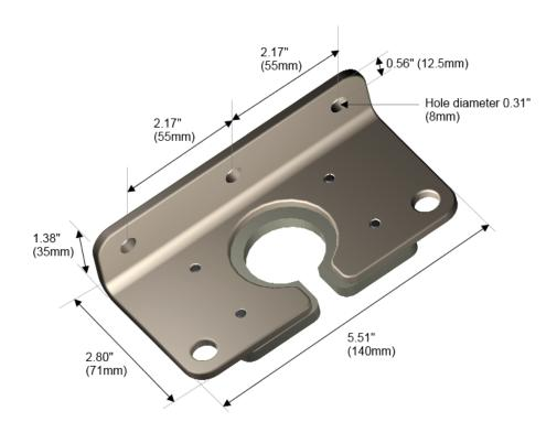
Bracket thickness 0.20" (5mm) Bracket material: powder coated aluminum
